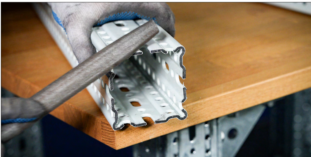
Treating cut edges with a hand file
